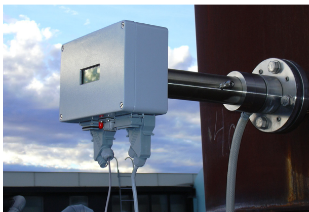
Figure 2. Transmitter unit of an in-situ TDLAS gas analyser.
